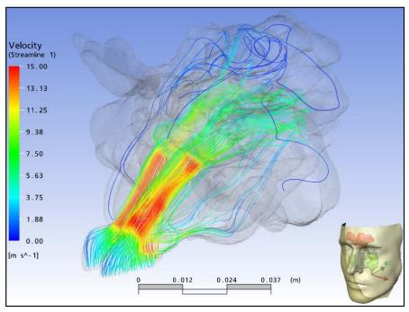
Visualization of inspiratory flow up to 16 m/s under laminar and turbulent conditions
