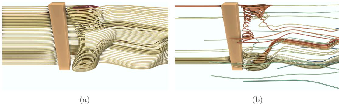
**Figure 3.4:** Comparison between a regular seeding approach with filtering (a) and an evolutionary seeding approach (b) to highlight a vortex using the same quality criterion for the filtering and evolutionary algorithm [143].
