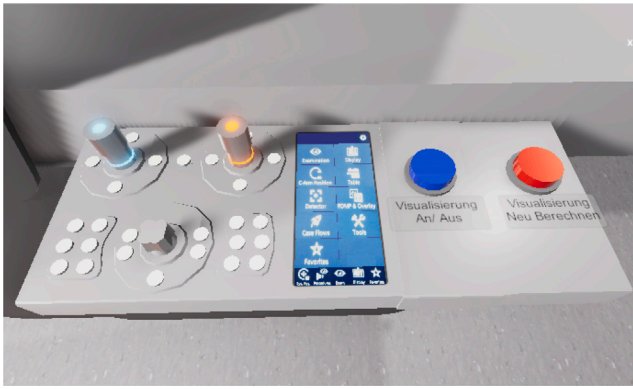
Fig. 5. The control panel for both C-Arms. The orange and blue control stick are used to rotate and move the Arms. The display is used to select specific position presets. The blue and red button are used to start and recalculate the radiation visualization.
