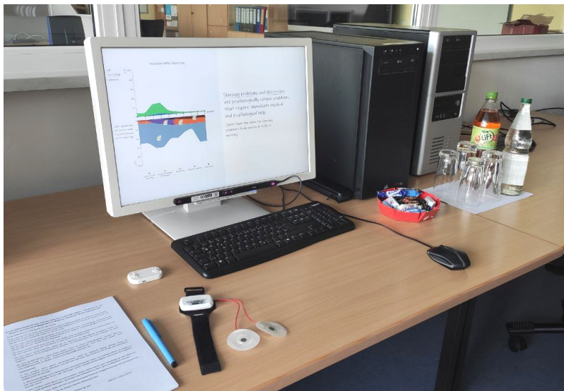
Figure 8.1: Experimental setup including EDA sensor, eye tracking device, questionnaires, and interactive slideshow prototypes in a lab of the Department of Simulation and Graphics.
