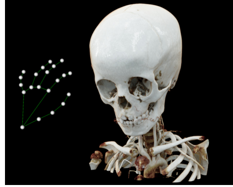
Figure 3: Visualization of the tracked hand using MediaPipe landmarks integrated into the interaction scene. The virtual hand provides visual feedback of the recognized hand pose and helps users understand the relationship between their hand configuration and the resulting interaction.
