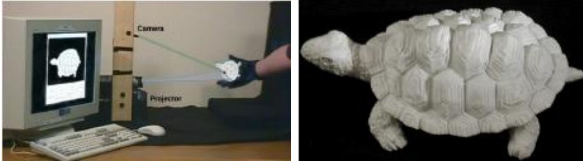
(a) Portable scanner device connected to the computer while fixed on the table (b) Close view of the object being scanned with portable scanner
