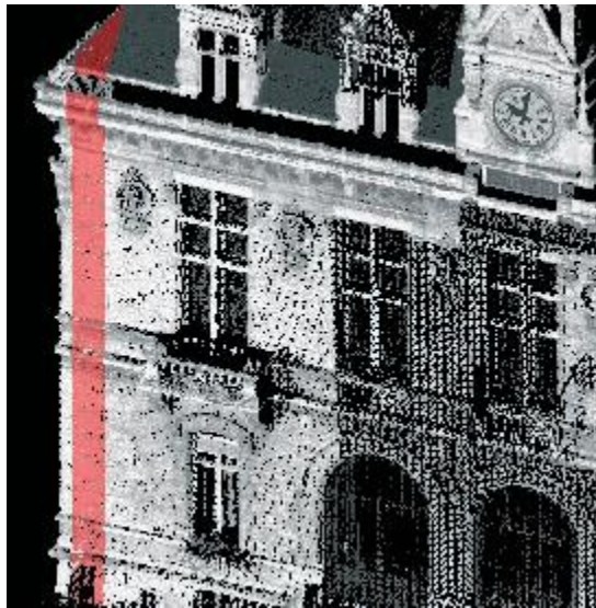
Figure 2.3: Point clouds of a building generated from a Time-of-Flight method [Gmb07]
