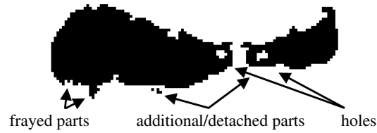
Figure 4: Example of a segmentation result suffering from frayed parts, holes, additional and detached parts.
