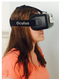
Figure 3.20: The Oculus Rift as an example for a binocular head-mounted display.
