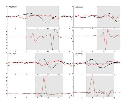
Fig. 2. Velocity profiles (top in each subplot) corresponding to pre- (black) and post-CRT (red) data, together with EGMs (bottom in each subplot) of  $EP_{elat}$  and  $EP_{llat}$  (black and red, respectively) for cases with septal flash. The dashed markers and grey area define the septal flash interval.
