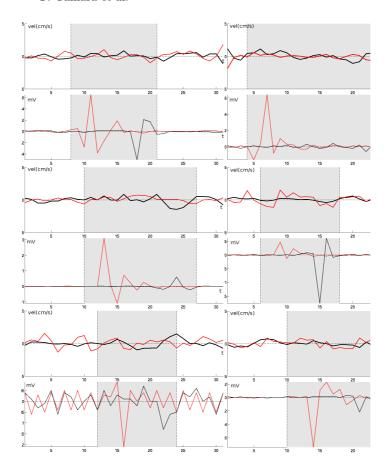
Fig. 3. Velocity profiles (top in each subplot) corresponding to pre- (black) and post-CRT (red) data, together with EGMs (bottom in each subplot) of  $EP_{elat}$  and  $EP_{llat}$  (black and red, respectively) for cases without septal flash. The dashed markers and grey area define the septal flash interval.
