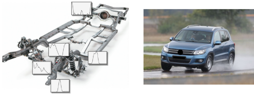
Figure 32: A test car equipped with more than 100 sensors.
