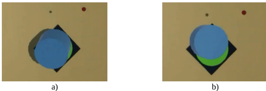
Figure 15: Placement test. Image a) shows the cylinder falling on its goal field. It collides with the ground while in a tilted orientation. The performed acceptance test at collision evaluates the target as not being correctly placed. In b) the target has settled on the ground in an acceptable position, but because no further test is performed, the placement is not accepted.
