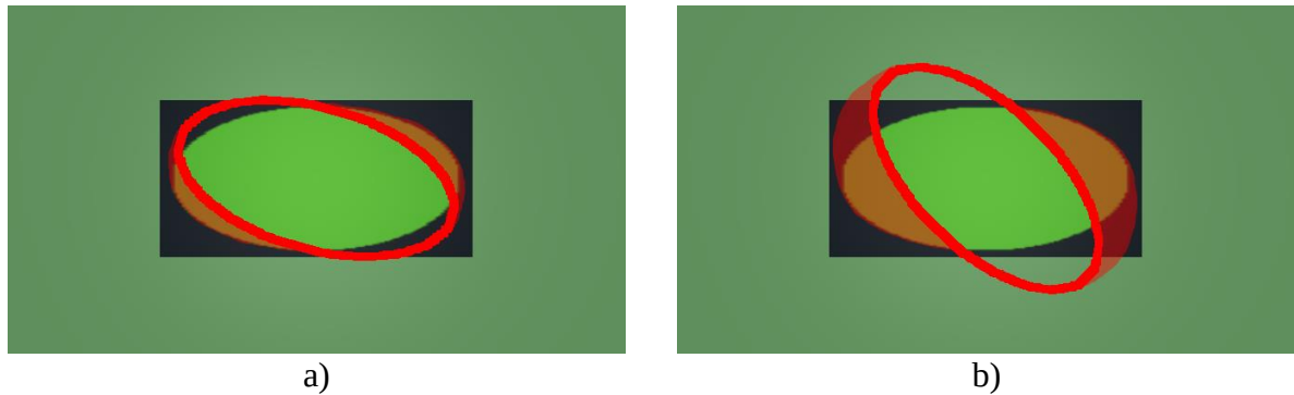
Figure 14: Tolerance limits for the target orientation (elliptic cylinder goal). An object is considered correctly placed, if it is not further rotated from the goal's orientation than the defined limit in both directions. The tolerated area for a clockwise rotation is marked in red. Limits for the preliminary study are 15° a) and for the final study 44° b).
