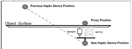
Figure 1: Training setup with Phantom. Figure 2: Resistance force is calculated by spring-damper simulation between device position and proxy position constrained outside of (or on) a surface. [9]
