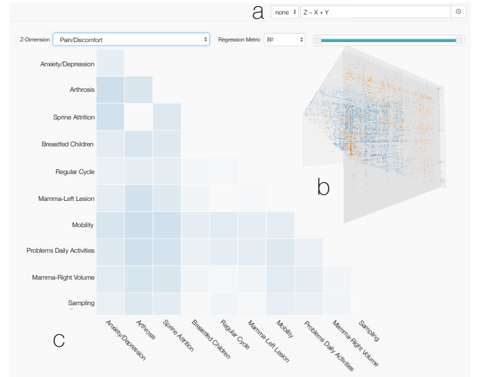
Fig. 2. Breast density data set loaded into our prototype. (a) Using the formula input, the user specifies the dependent feature and calculation rules. (b) 3D heat map showing values above the matrix diagonal as overview. The values of the currently selected slice are mirrored and represented as orange data points on the slicing plane. (c) 2D heat map of the selected slice for feature Pain/Discomfort .
