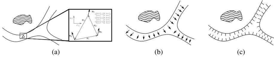
**Fig. 2.** Overview of the *ConFIS* method. In the first step, the curvature tensor per triangle is determined, see (a). This is used to calculate the principle curvature directions per vertex, see (b). Afterwards, the streamlines are determined, see (c).
