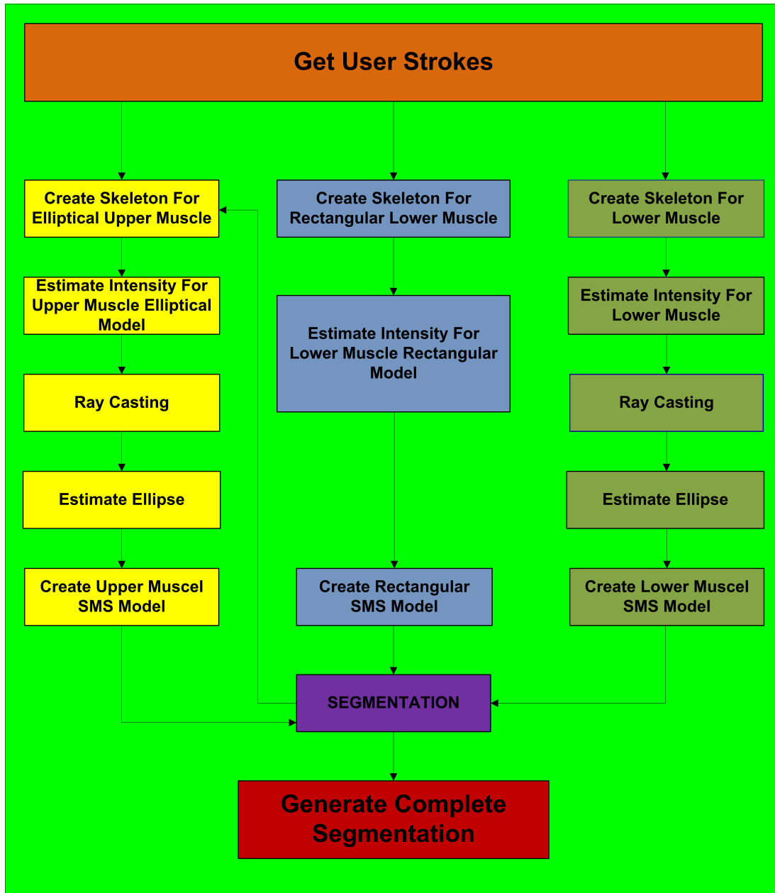
Figure 4.4: Work flow diagram of the segmentation process.
