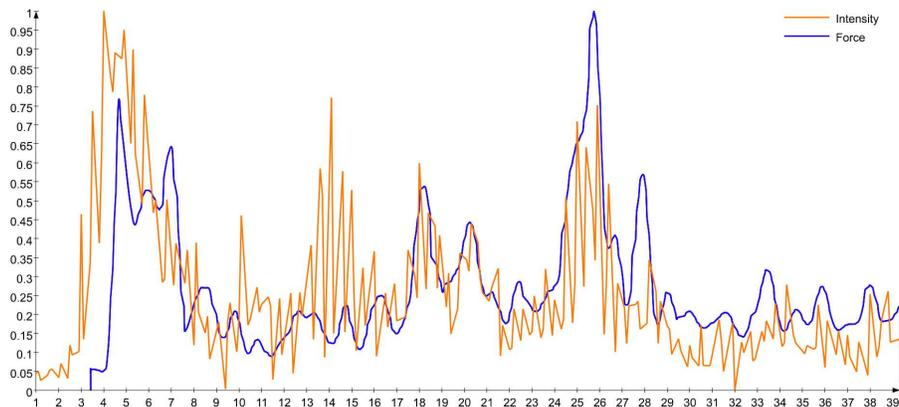
Figure 5: Normalized forces (blue) and normalized, averaged intensities (orange) during insertion with constant velocity through a lumbar pedicle (Fig. 1).
