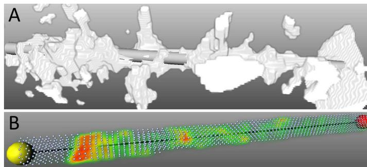
Figure 4: (A) Remaining intensity values after image subtraction and thresholding with a high number of segmentation artifacts. (B) The drill was inserted from the yellow to the red sphere. The red area on the left is the result of high intensity values: It depicts the position of the vertebral corticalis, which is harder than the vertebral body.
