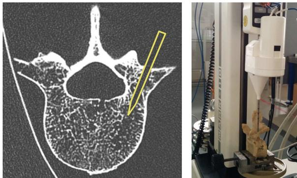
Figure 1: *Left*: 10 s Dyna-CT scan with highlighted insertion path for a conserved lumbar vertebrae. *Right*: Experimental setup where forces are measured during automatic drill insertion with constant velocity of 2 mm per second.
