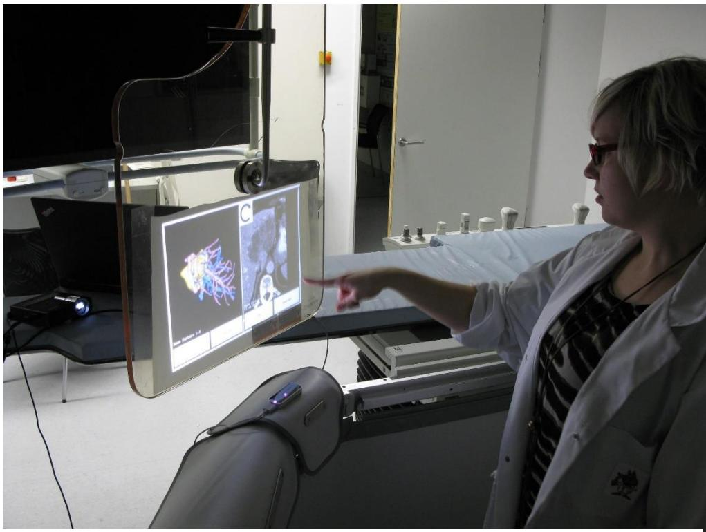
**Figure 2:** Setup of our prototype. The projector on the left is projecting the viewer software onto the radiation shield in the middle. Below the acrylic glass, the LMC is placed to recognize hand and finger gestures for the interaction.
