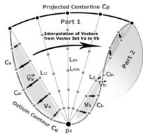
(b) Interpolation scheme for one of the two surface parts
