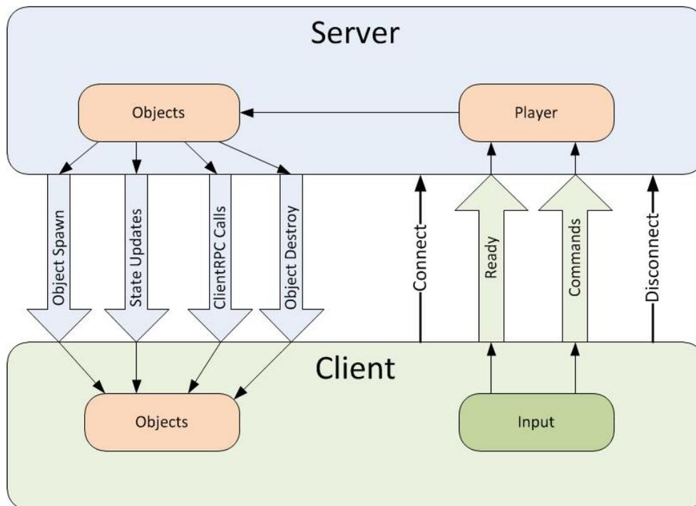
Figure 4.3: The diagram illustrates how information can be synchronized between the server and clients.
