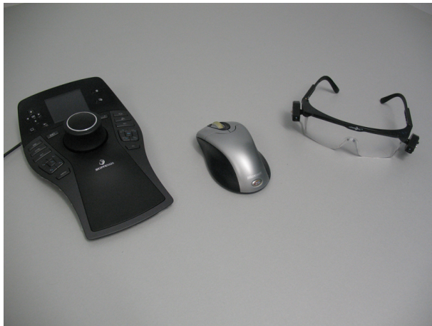
Figure 18: The different interaction devices: (left) SpacePilot Pro, (middle) standard mouse, and (right) head tracking.
