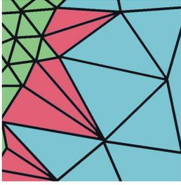
**Fig. 11** Due to a rapid change in size between small (green) and big (blue) triangles, degenerated triangles (red) are created.
