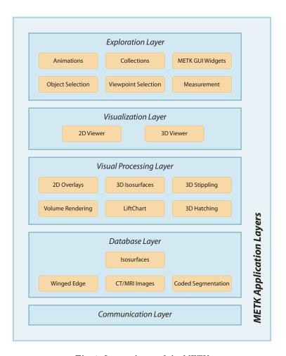
${\bf Fig.\,1.}$  Layer schema of the METK.
